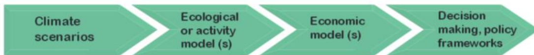
Figure 1 Schematic of an end-to-end assessment strategy, also referred to as a ‘feed forward approach’, for a local/regional climate change impact assessment. (Source: Winkler et al. 2011)
